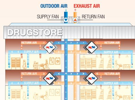
The air quality in a building is one of the main factors for internal comfort. The air must be continuously changed to maintain safe conditions. This process wastes energy, which can be recovered by installing a plate heat exchanger. Let's examine a drugstore with an area of 1235 m<sup>2</sup>, and an average density of 310 people. To change the air, 10,000 m<sup>3</sup>/h of fresh air, is needed. The example shows a system with our air to air plate heat exchanger:
